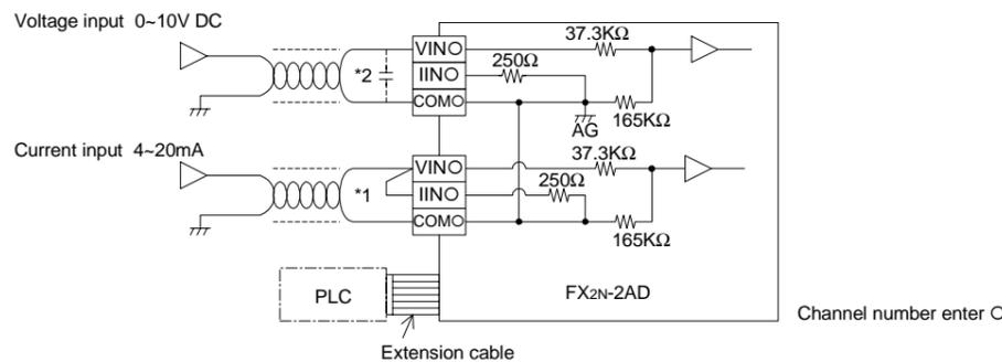
\*1 The FX<sub>2N</sub>-2AD cannot have 1 channel as an analog voltage input and one channel as current input because both channels use the same offset and gain values. For current input please short circuit VIN and IIN as shown in the diagram.
