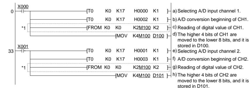
Analog to digital conversion execution input of CH1:X000
